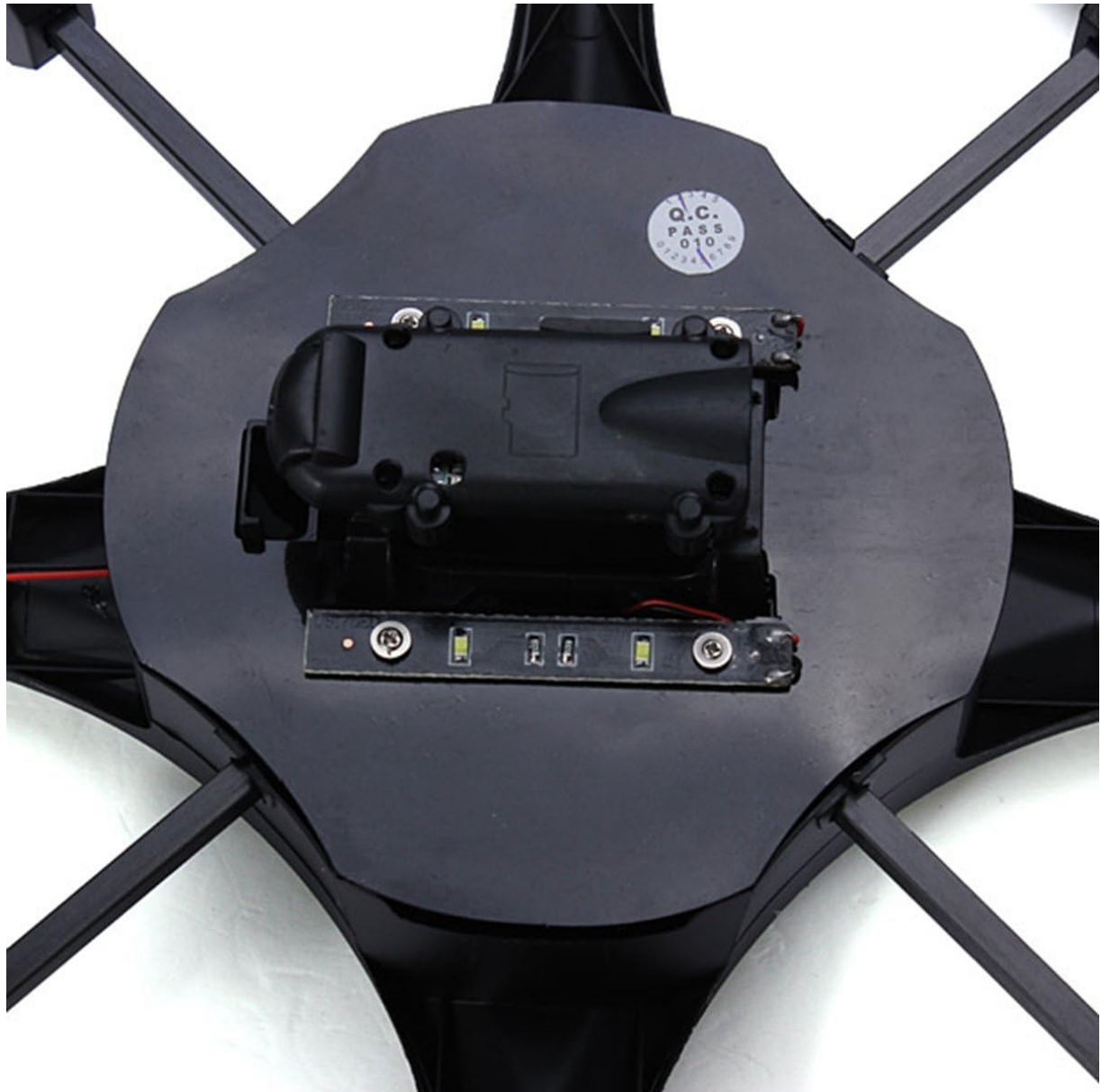
Image: Underside view of the quadcopter, highlighting the camera and LED lights.
