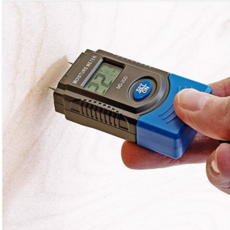
Figure 3: The Draper 43618 Moisture Meter being used to measure moisture on a light-colored wooden surface. The meter is held firmly, ensuring the probes are inserted into the material, and the display shows a reading of "7.2%".
