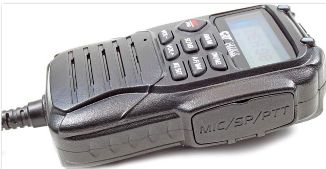
Figure 3.3: Side view of the CRT Mike microphone, highlighting the speaker grille and the MIC/SP/PTT port for external connections and the Push-To-Talk button.
