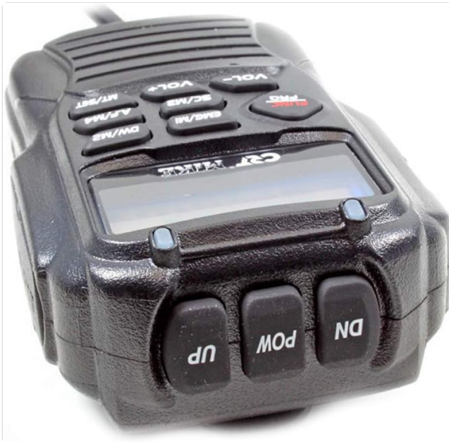
Figure 3.4: Top view of the CRT Mike microphone, displaying the UP, POW (Power), and DN (Down) buttons for channel selection and power control.
