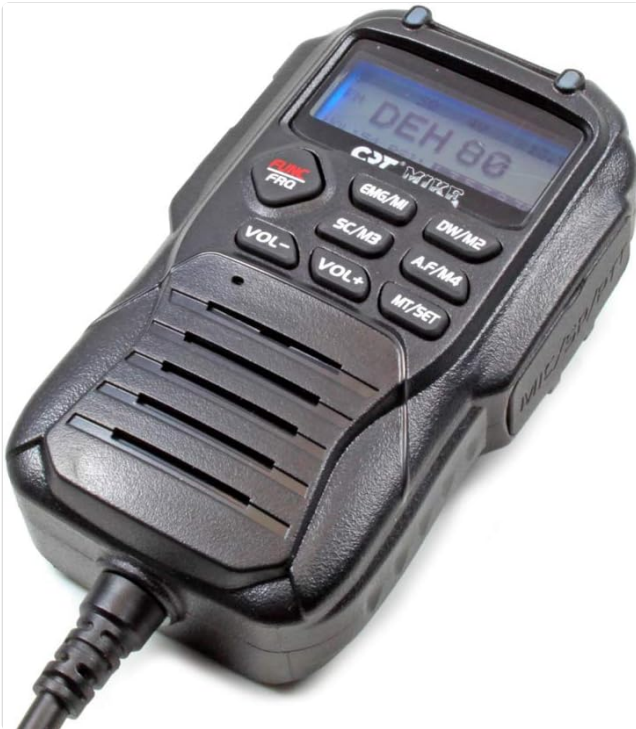
Figure 3.2: Front view of the CRT Mike microphone, showing the display screen and primary control buttons such as MEM, FRQ, VOL-, VOL+, SC/M3, AF/M4, EMG/M1, DW/M2, and MT/SET.
