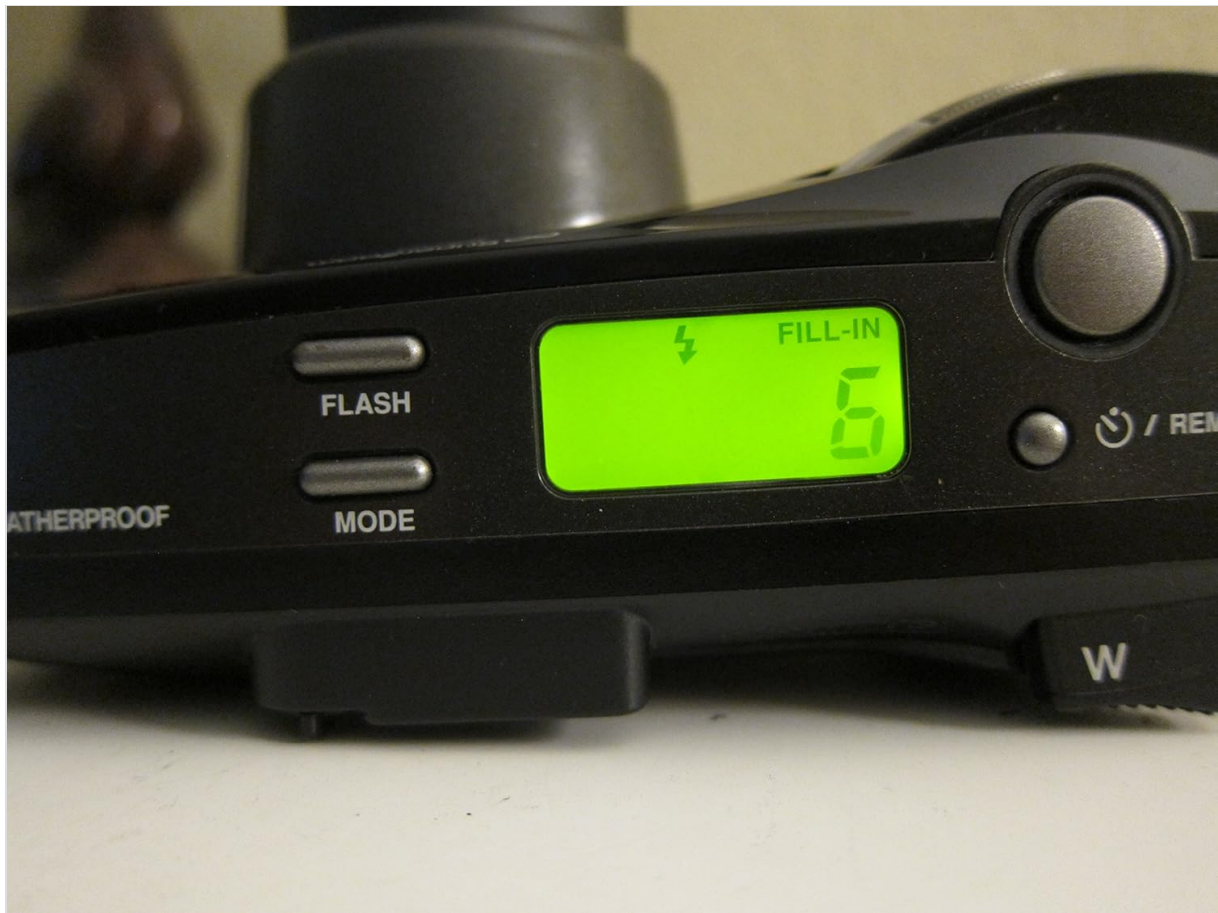
Figure 6: Close-up of the LCD display, showing the 'FILL-IN' flash mode indicator.
