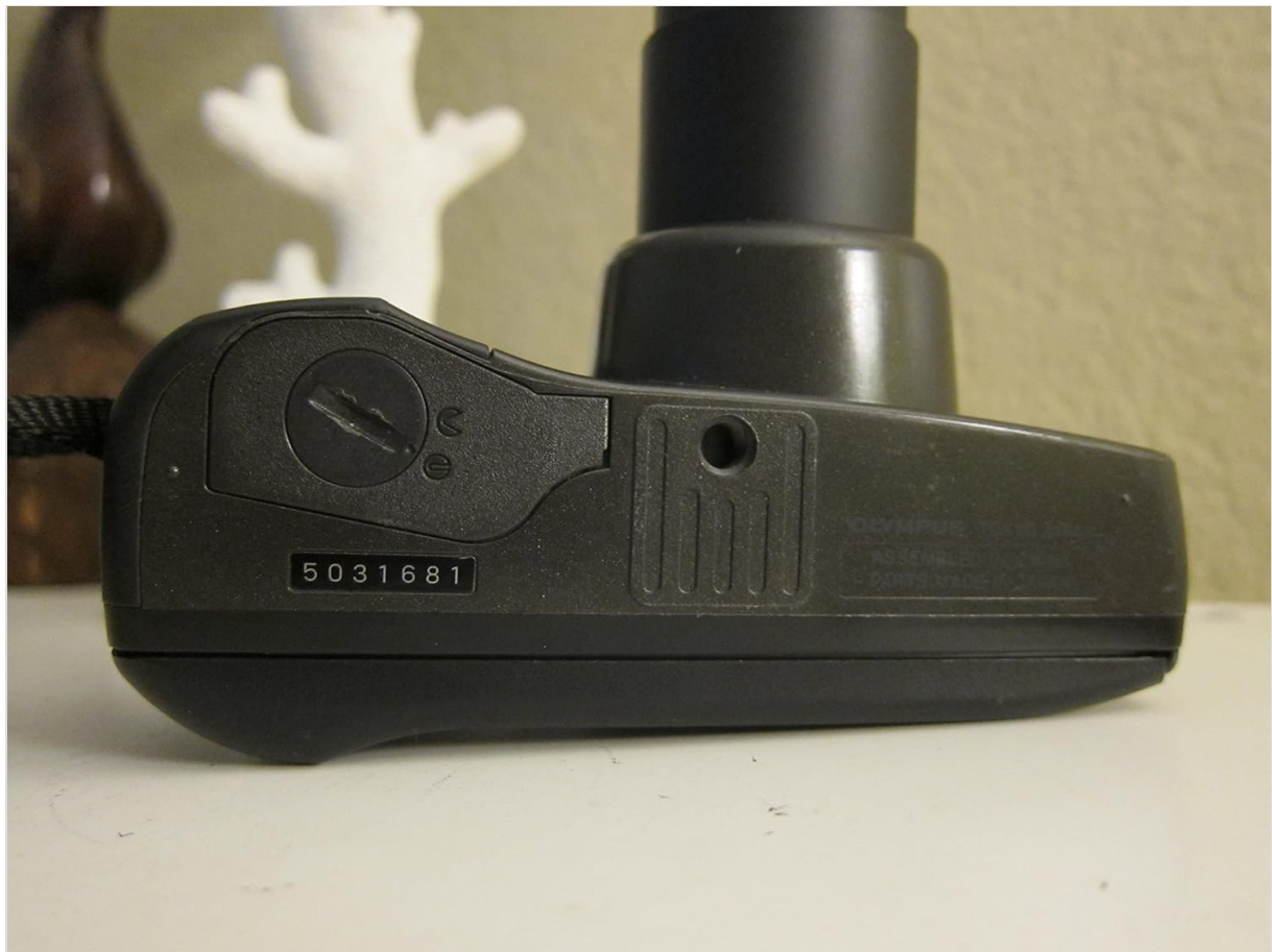
Figure 1: Bottom view of the camera, illustrating the battery compartment and tripod mount.
