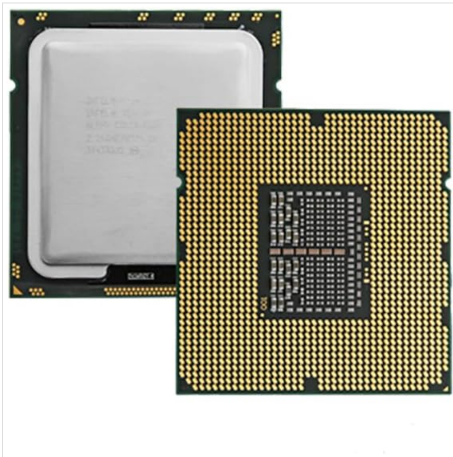
Figure 1: Intel Xeon E5-2640 v3 Processor. This image displays two views of the processor: the top side with the integrated heat spreader (IHS) and the bottom side revealing the LGA 2011-3 pin array.
