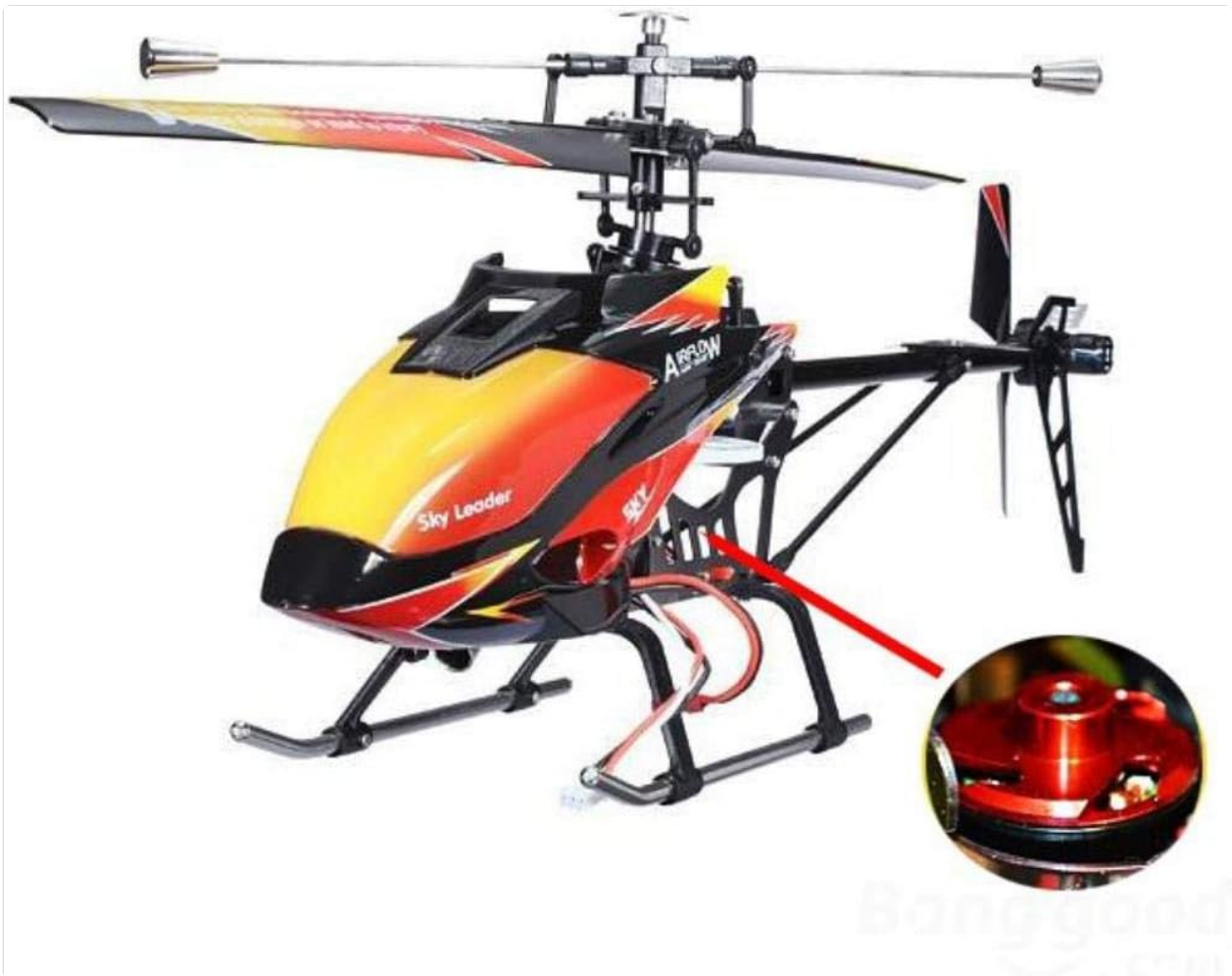
Image 1.1: Front view of the WLtoys V913 Brushless RC Helicopter, showcasing its main rotor, tail rotor, and landing skids.
