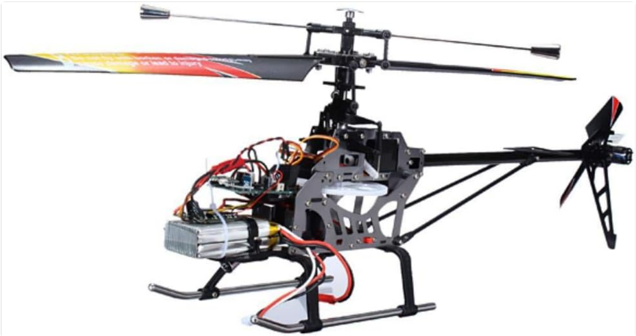
Image 4.1: Side view of the helicopter showing the battery compartment and internal wiring. The battery is secured with a strap.
