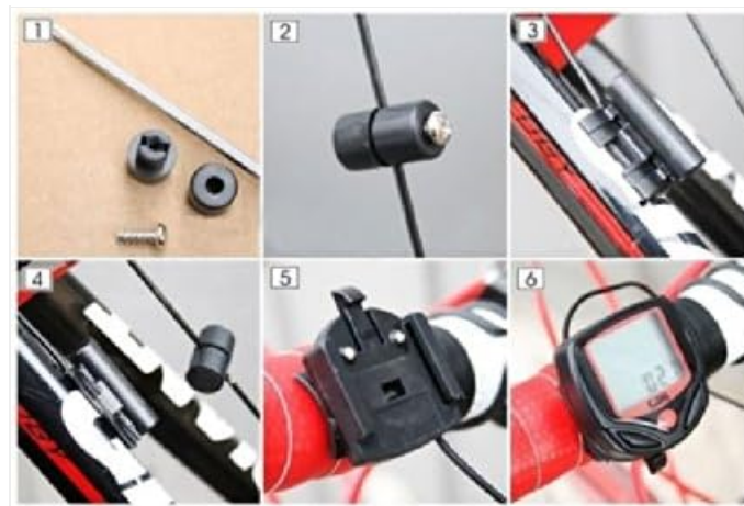
Image: A six-panel image illustrating the step-by-step installation process for the cycle computer, including sensor, magnet, and main unit mounting.
