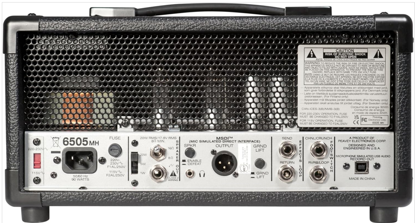
Image: Rear panel of the Peavey 6505 MH amplifier. This view highlights the various input and output jacks, including the speaker output, impedance switch, MSDI, effects loop, and USB port.
