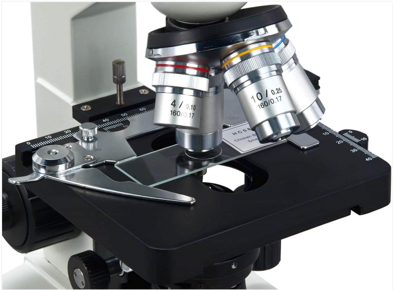
Figure 2: Close-up view of the revolving nosepiece with objective lenses and the mechanical stage with stage clips. This illustrates the components involved in selecting magnification and positioning the specimen.
