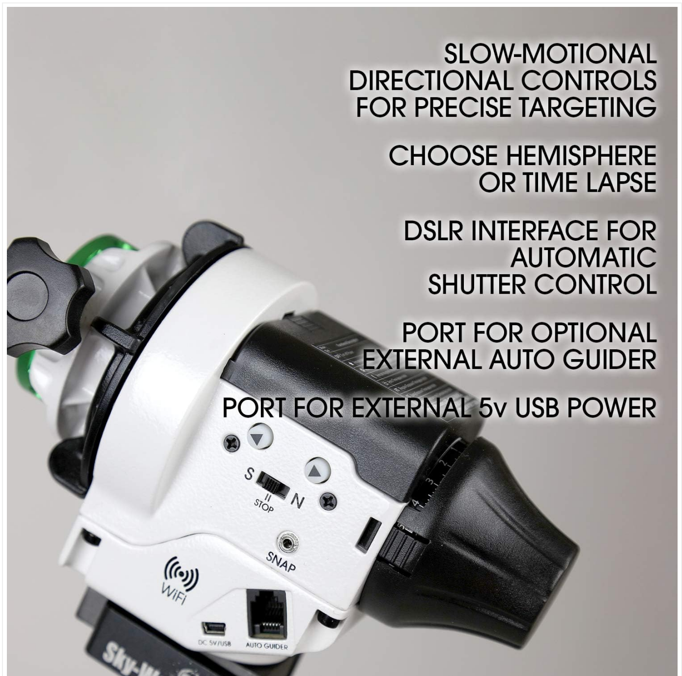
Figure 5.1: Side view showing various ports and controls.
