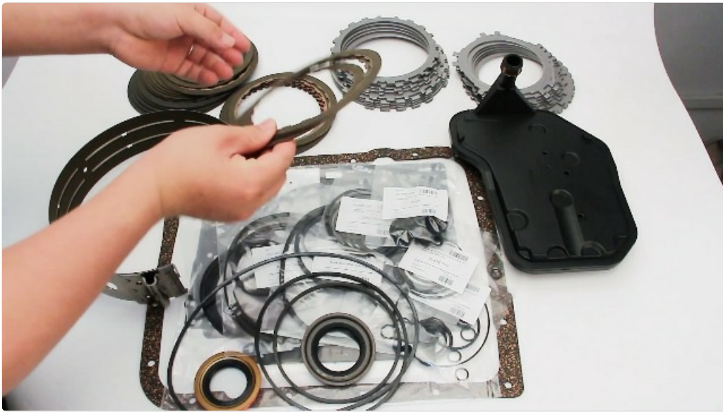
Image: A visual representation of the various components included in a typical 4L60E transmission rebuild kit, such as friction plates, steel plates, bands, seals, and the transmission filter.
