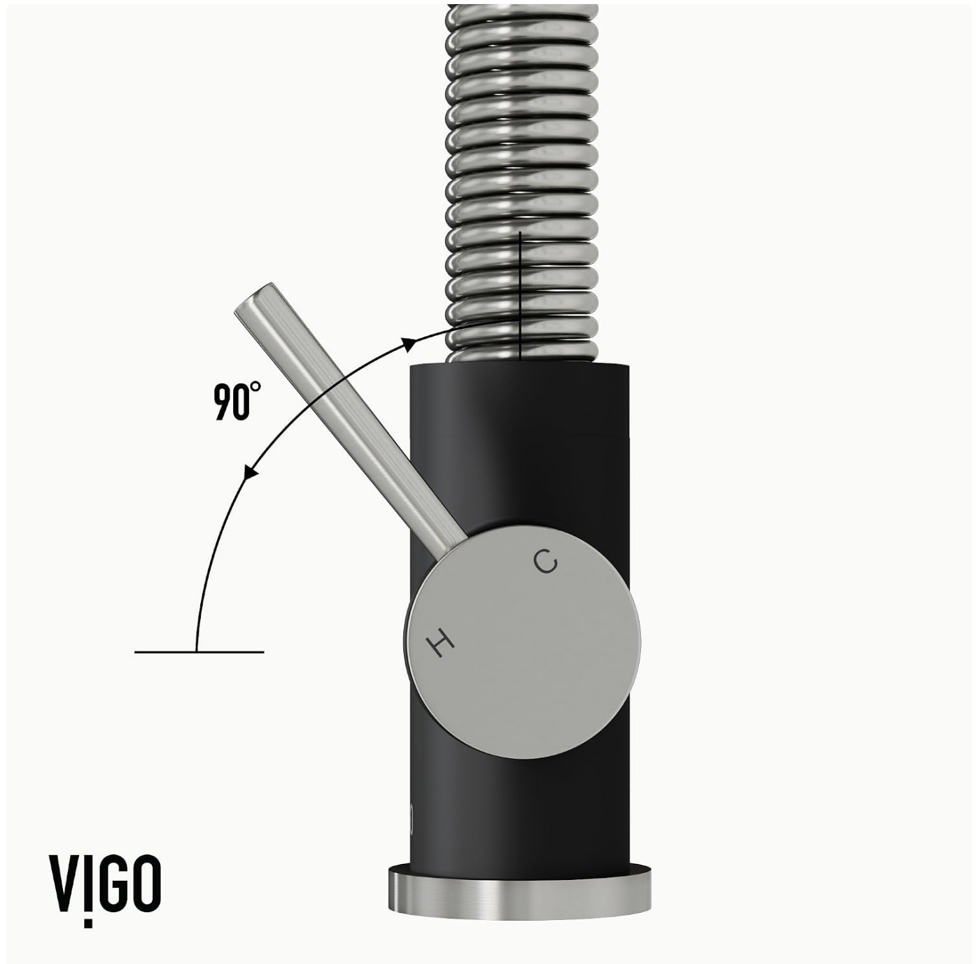
Image 6.1: Faucet handle operation for temperature and flow control.
