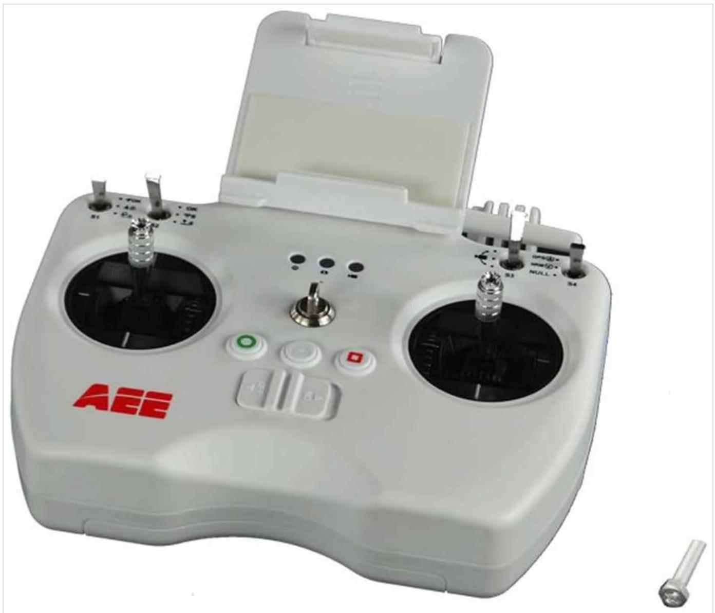
The AEE Y08F Radio Controller is a white, ergonomic device designed for controlling the AEE Toruk AP10 drone. It features two main joysticks for flight control, various toggle switches for mode selection and camera functions, and a central power switch. A foldable smartphone holder is integrated at the top for FPV (First Person View) monitoring.
