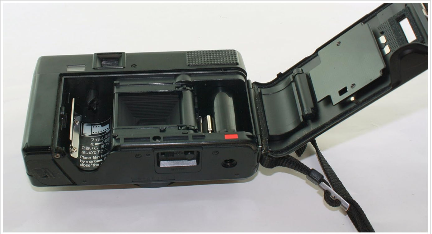
Figure 2.2: The Nikon L35AF with its back cover open, revealing the film chamber and take-up spool for film loading.
