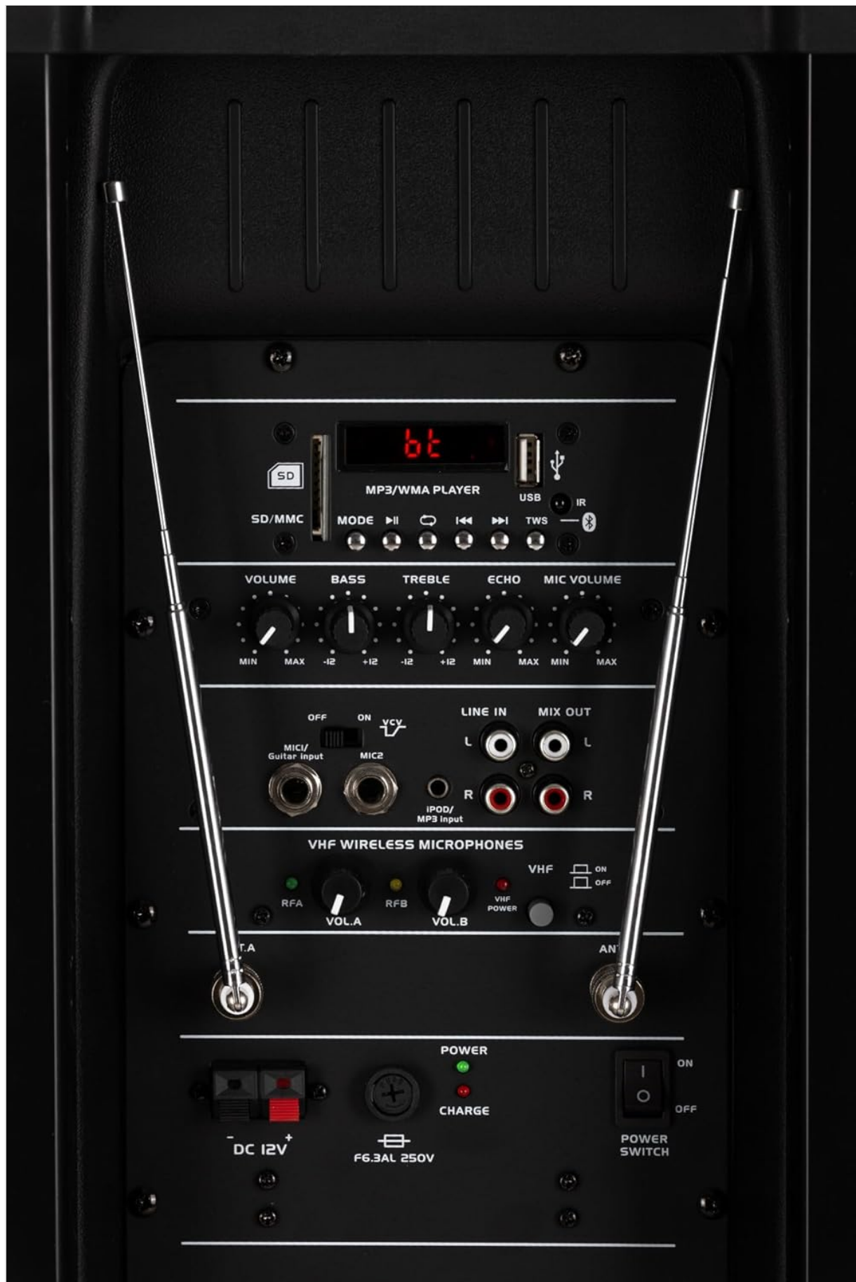
Image 4.3: A closer look at the MP3 player section, EQ controls, and microphone inputs.
