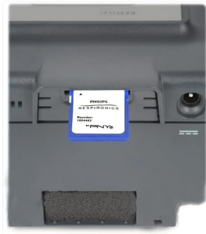
Image 2: The Respironics System One Data Card partially inserted into the dedicated slot of a Philips Respironics CPAP machine, demonstrating the correct orientation for installation.
