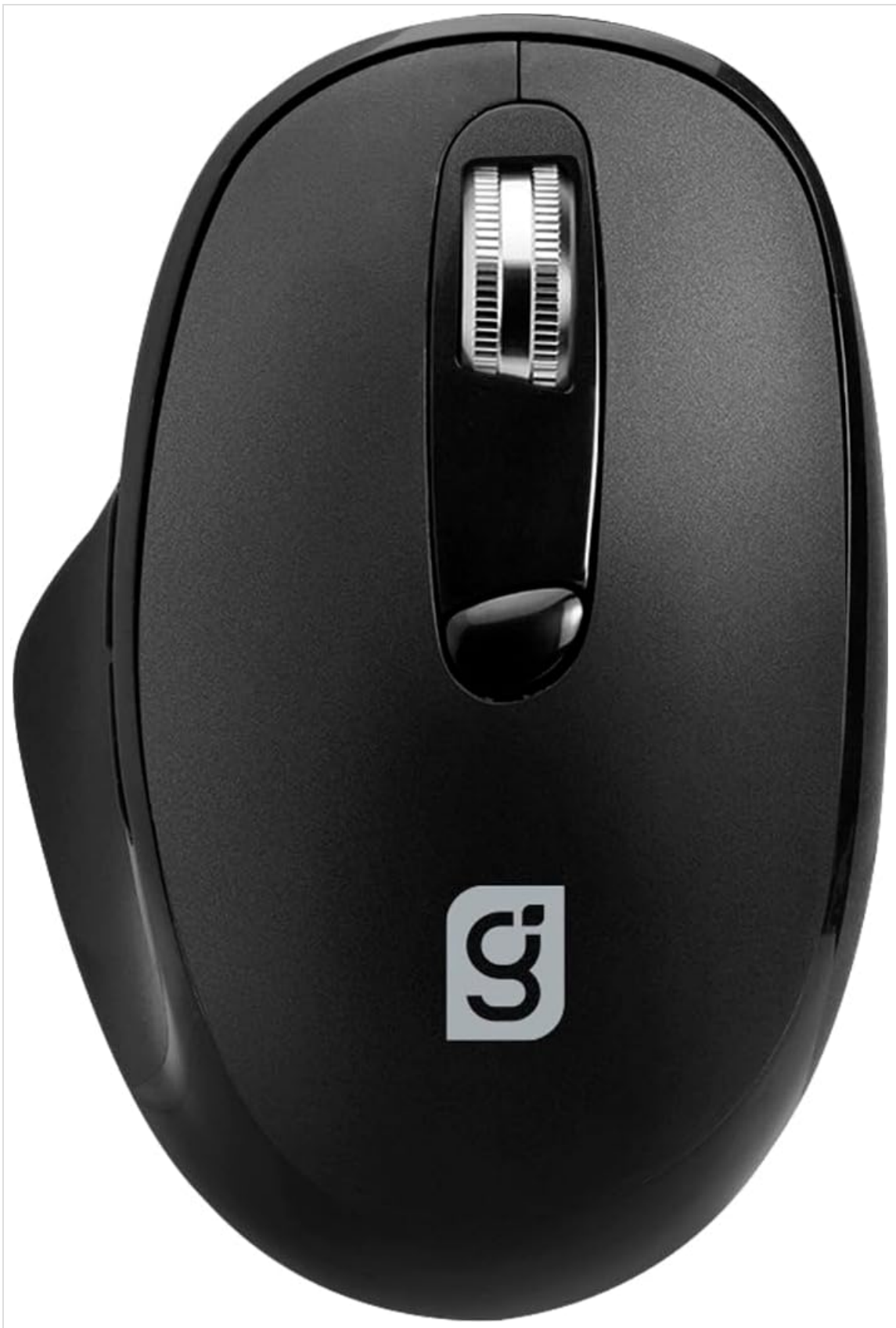
Figure 3.1: Top view of the Green Leaf 18-8846BK Wireless Mouse, showing the left and right click buttons, scroll wheel, and DPI button.
