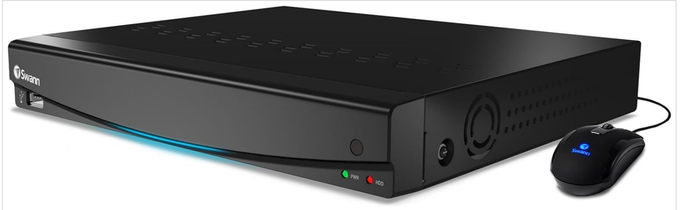
Figure 3.1: The Swann DVR unit with the USB mouse connected. The front panel displays power and hard drive activity indicators, essential for monitoring system status.
