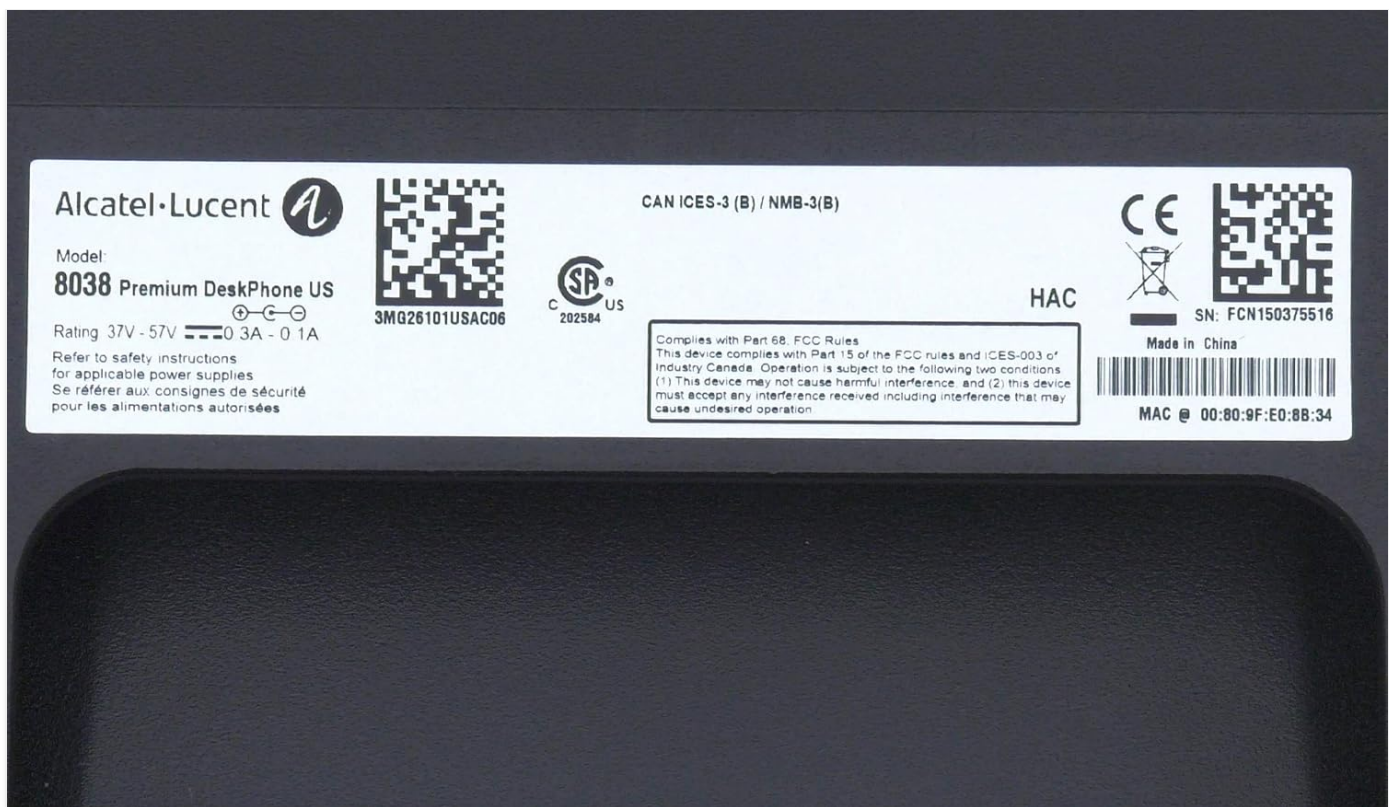
Figure 2: Rear label of the Alcatel-Lucent 8038 Premium DeskPhone, showing model and serial number.
