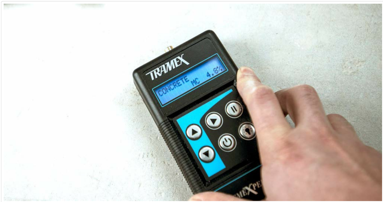
Figure 1: Close-up view of the Tramex CMEX2 CMEXpert II digital display. The screen clearly shows 'CONCRETE MC 4.8%', indicating a moisture content reading of 4.8% in concrete. The device features several control buttons for navigation and operation.
