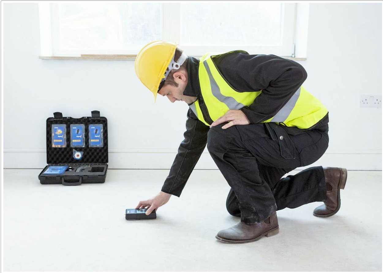
Figure 2: A construction worker, wearing a hard hat and safety vest, kneels to use the Tramex CMEX2 CMEXpert II moisture meter on a concrete floor. The device is placed flat on the surface to take a reading. In the background, a carrying case with additional probes and equipment is visible.
