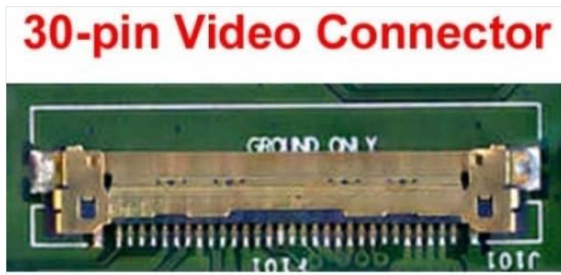
Image 4: A clear close-up of a 30-pin video connector, providing a detailed view for identification and confirming compatibility with the replacement screen.
