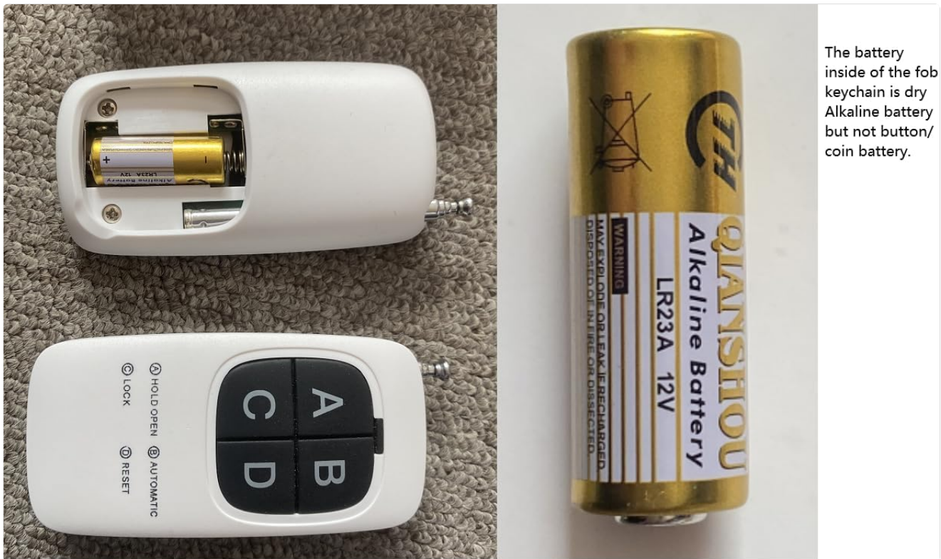
Figure 3.2: The remote control unit, showing its four buttons (A, B, C, D) for various functions and the battery compartment for an LR23A 12V alkaline battery.
