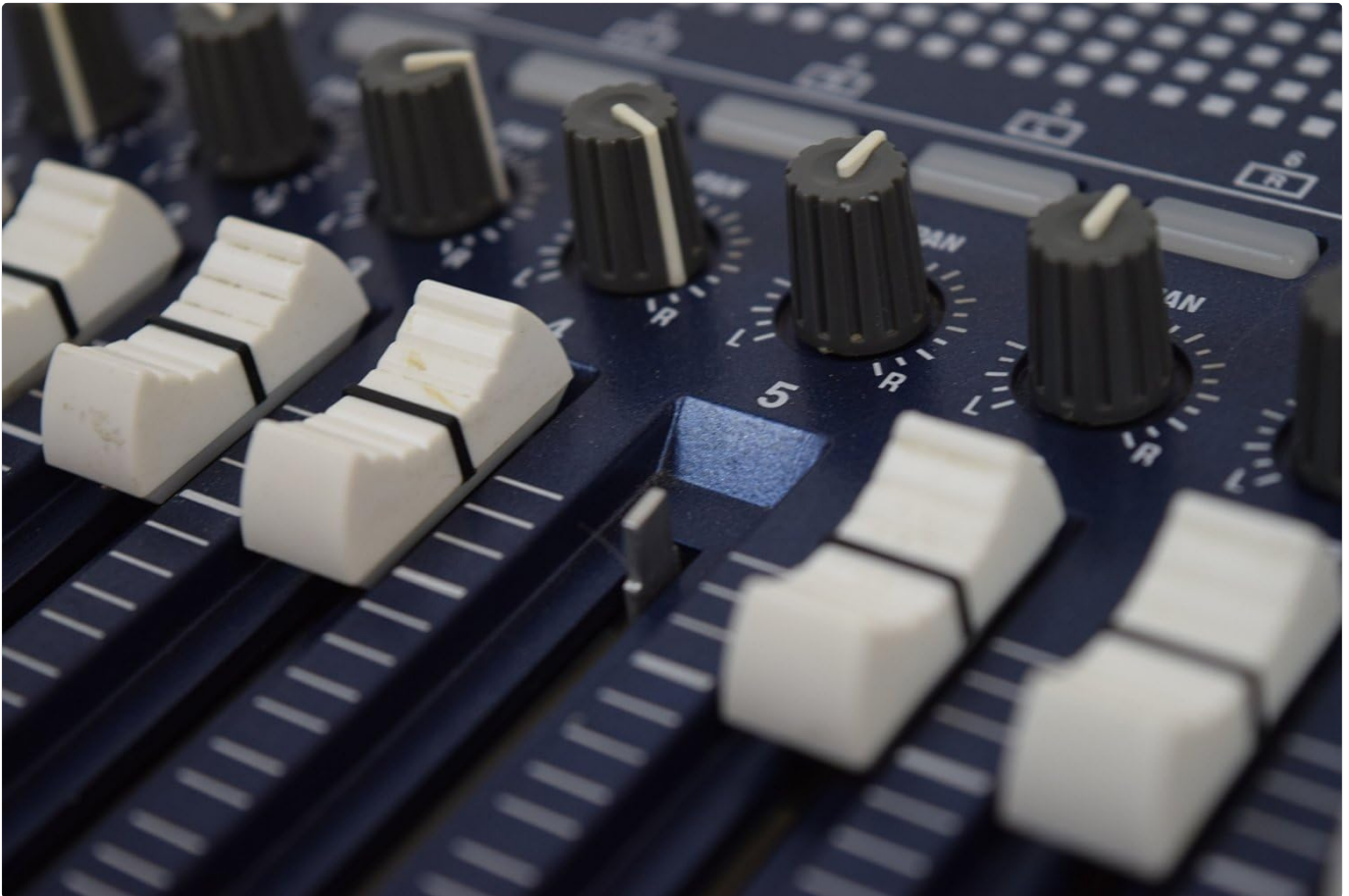
Figure 2: Detail of the mixing console section. This image highlights the faders and rotary knobs used for adjusting levels, pan, and EQ settings for individual channels during the mixing process.
