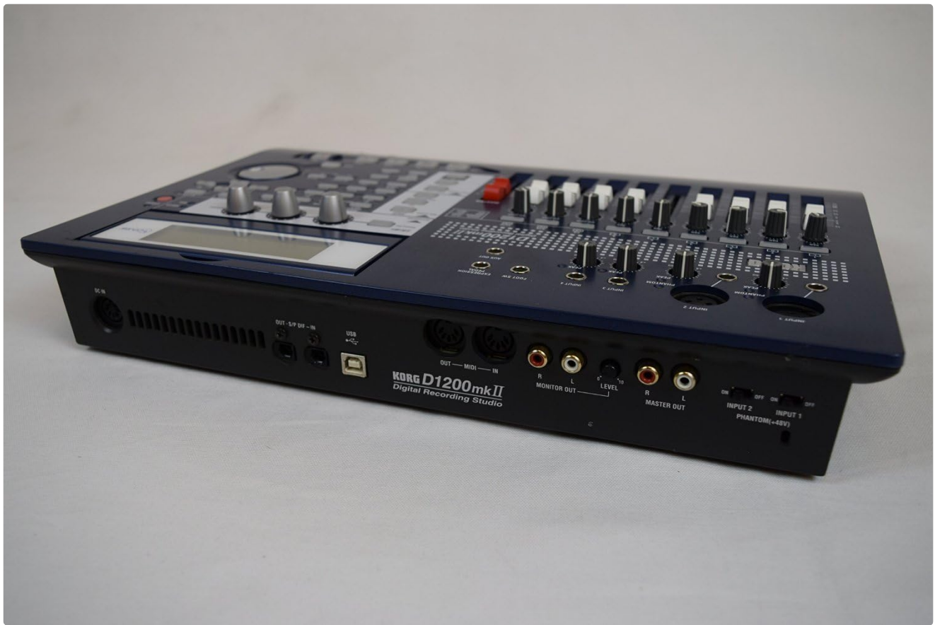
Figure 1: Rear panel connections of the Korg D-1200 MK2. This image displays the DC IN port for power, S/PDIF digital input/output, USB port for computer connection, MIDI IN/OUT, Monitor Out (L/R), Master Out (L/R), and Input 1/2 with phantom power switches.
