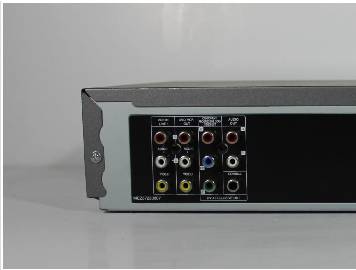
This image displays the rear panel of the JVC HR-XVC15, highlighting the VCR IN (Line 1), DVD/VCR OUT, Component/Progressive Scan Video OUT, and Audio OUT connections, along with Coaxial and DVD Exclusive Out ports.
