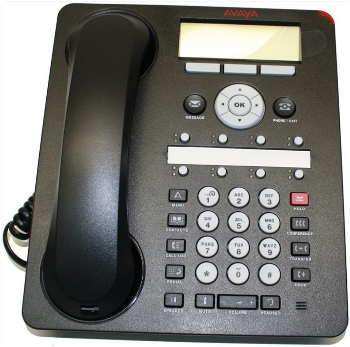
Figure 1: Top-down view of the Avaya 1608-I IP Phone, showing the handset, display, and keypad layout.
