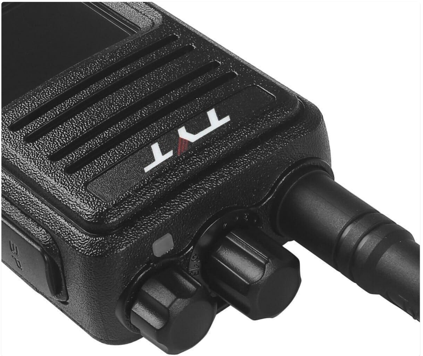
Figure 3.3: Top view of the TYT MD-380, illustrating the channel-selecting knob, power/volume knob, and antenna connection point.
