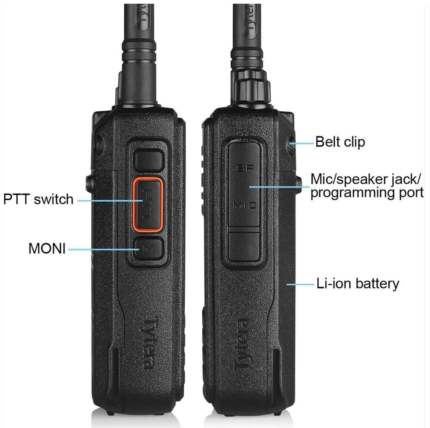
Figure 3.2: Side view of the TYT MD-380, highlighting the PTT switch, MONI button, mic/speaker jack (also used for programming), belt clip, and Li-ion battery compartment.
