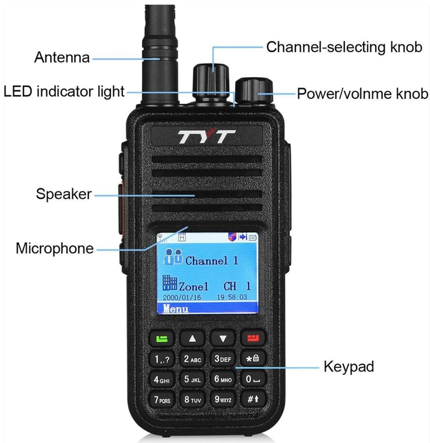
Figure 3.1: Front view of the TYT MD-380 with key components labeled, including the antenna, LED indicator light, channel-selecting knob, power/volume knob, speaker, microphone, and keypad.
