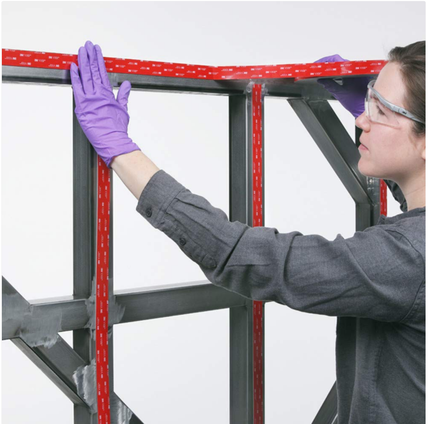
Image: A person wearing gloves and safety glasses applies a strip of 3M VHB tape to a metal frame, demonstrating the application process for structural bonding.
