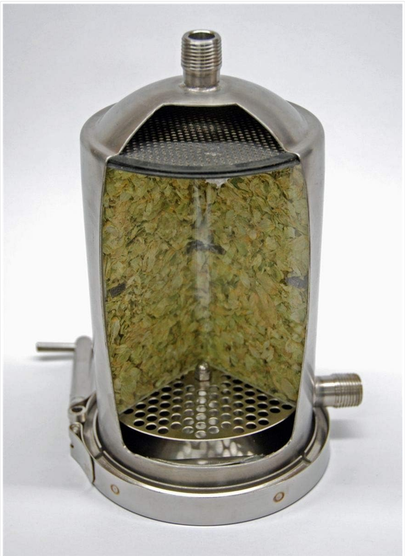
Figure 3: Cutaway view illustrating the internal chamber filled with hops, demonstrating the flow path through the unit.
