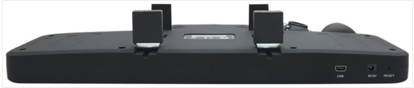
Figure 3.3: Bottom view of the M1000, showing the USB port, DC 5V power input, and reset button.
