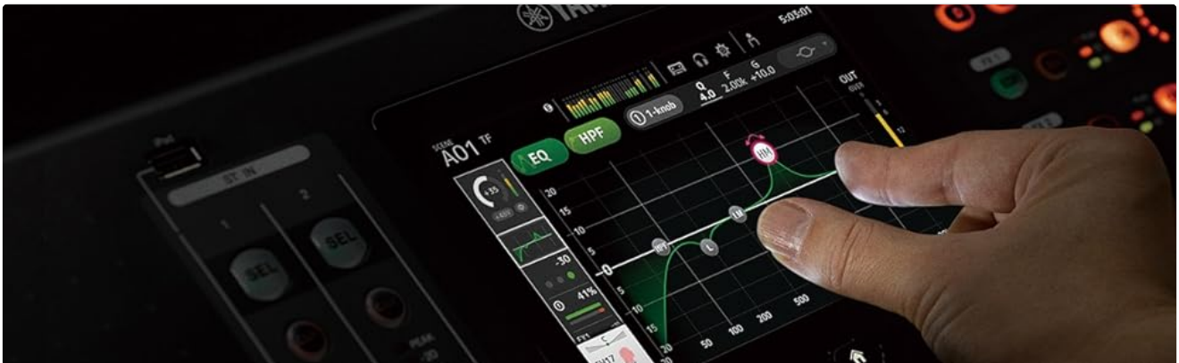
Figure 3: A close-up view of the TF3's touchscreen, demonstrating the intuitive graphical interface for adjusting equalization parameters.
