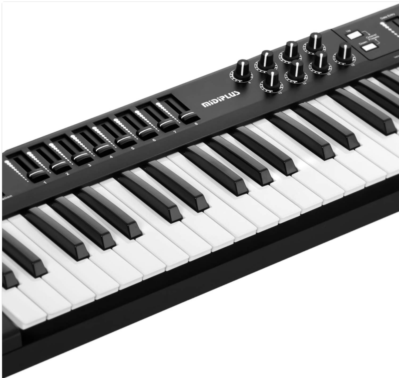
Figure 5.1: Close-up view of the eight assignable sliders and eight rotary encoders on the Midiplus Origin 62.
