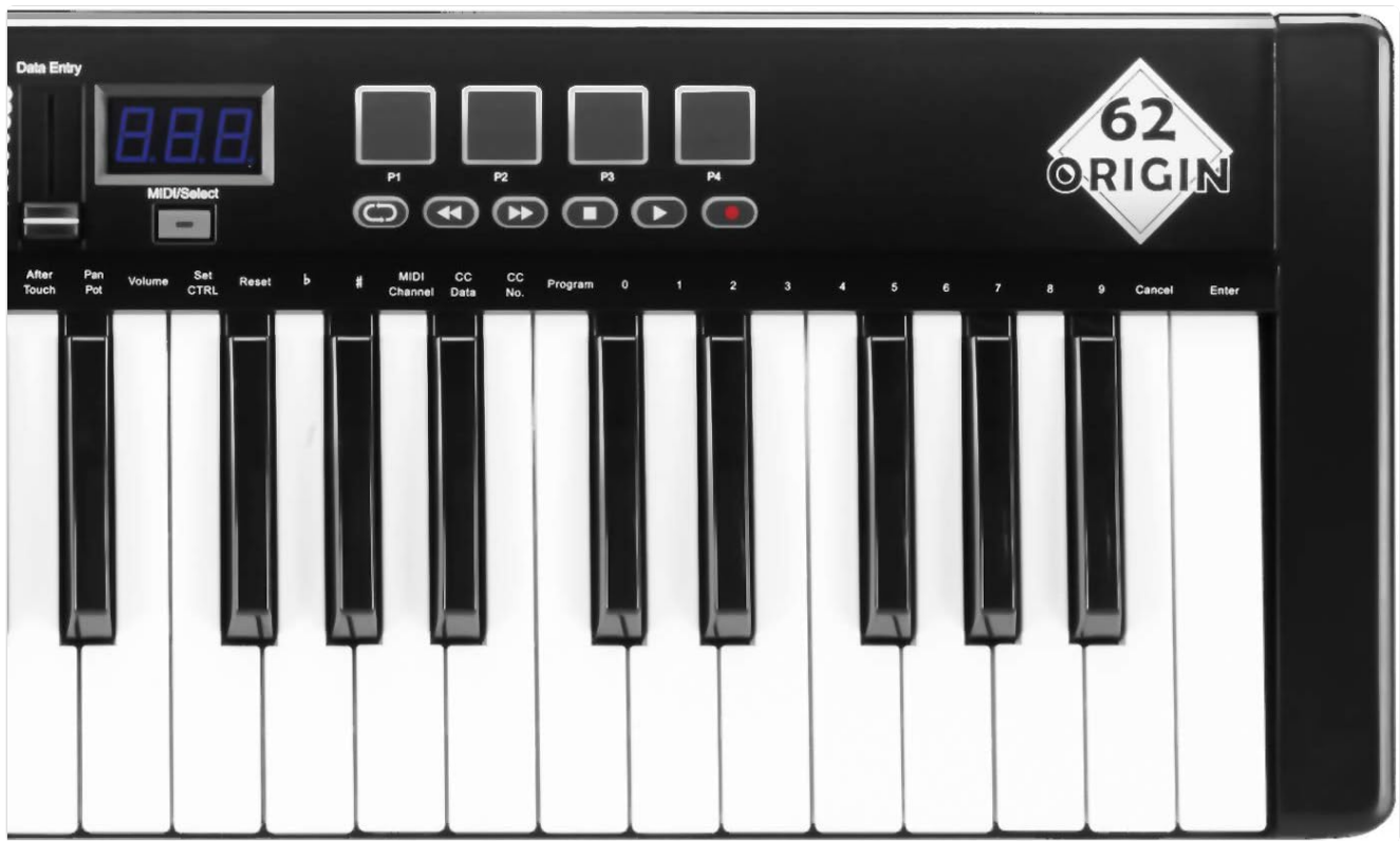
Figure 2.2: Close-up view of the data entry display, trigger pads (P1-P4), and transport controls on the Midiplus Origin 62.
