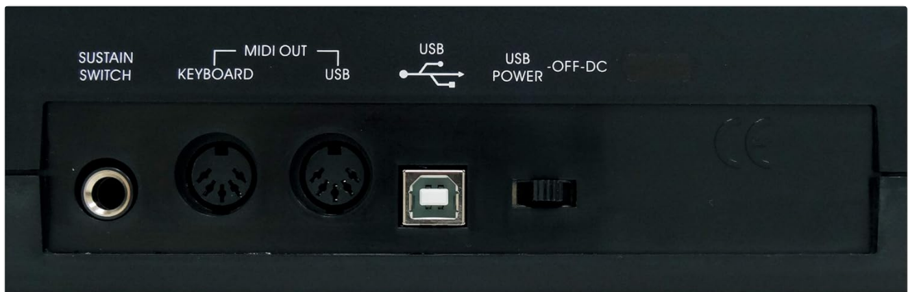
Figure 2.3: Rear view of the Midiplus Origin 62, showing the Sustain Switch input, MIDI Out port, USB port, and power switch.
