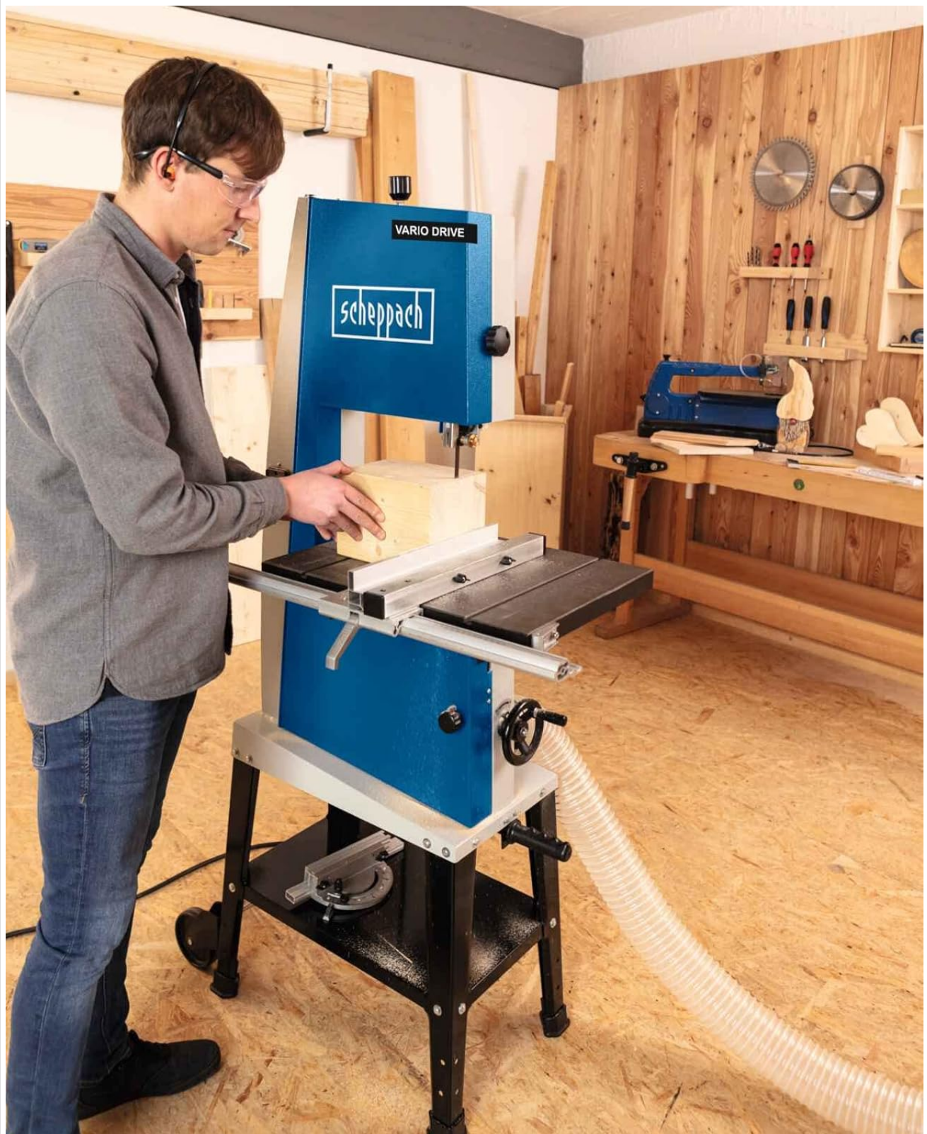
Figure 4.2: Connecting a dust extraction hose to the band saw for cleaner operation.
