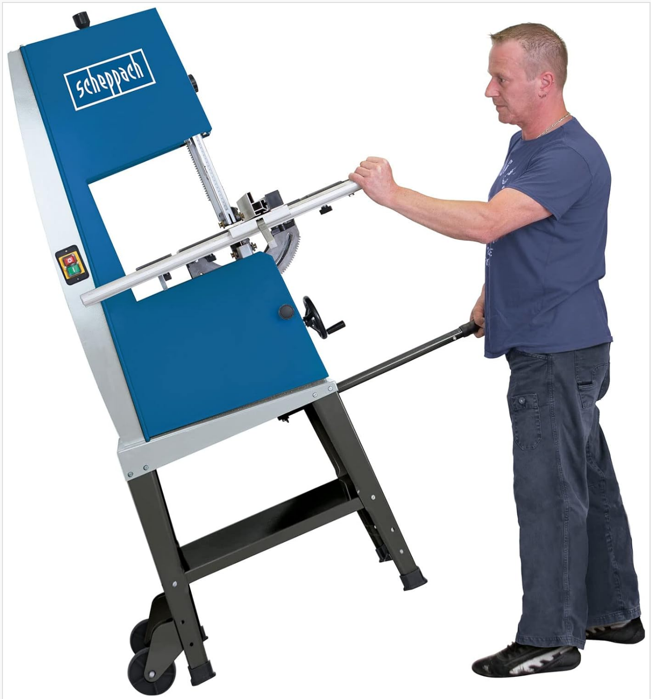
Figure 4.1: The integrated wheels and handle allow for easy tilting and movement of the band saw.
