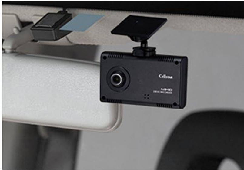
Figure 3.2.1: Drive recorder mounted on the windshield, providing a clear view of the road.
