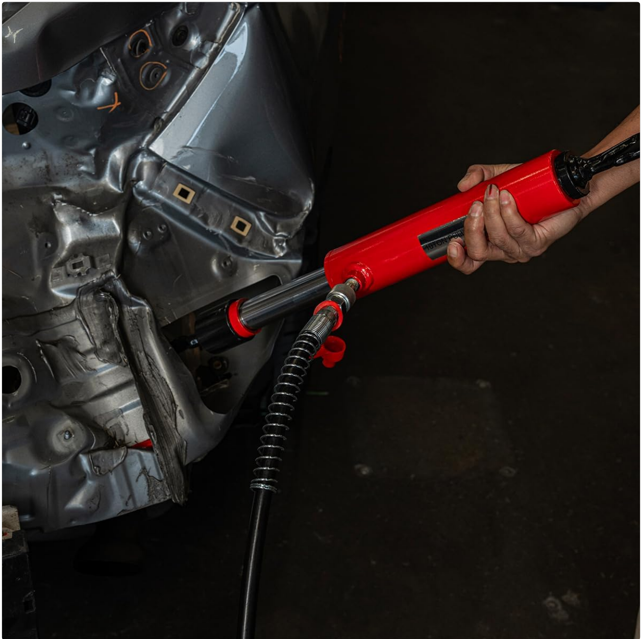
Figure 5: Ram used for straightening a metal component.
