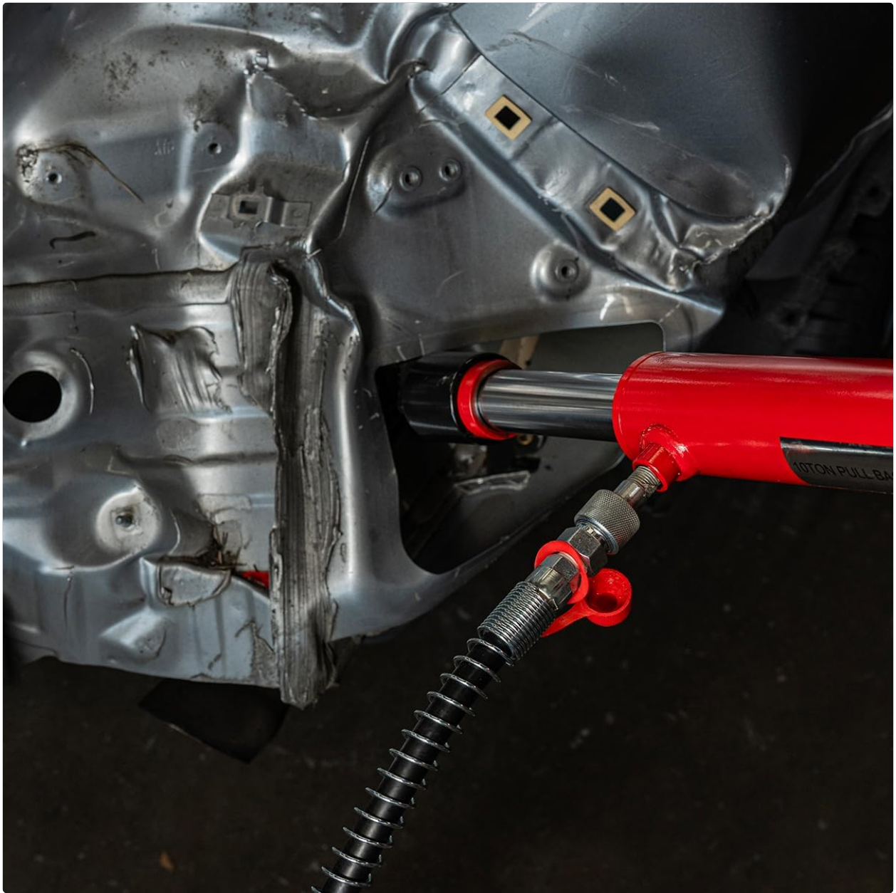
Figure 4: Ram applying pulling force to a vehicle frame.
