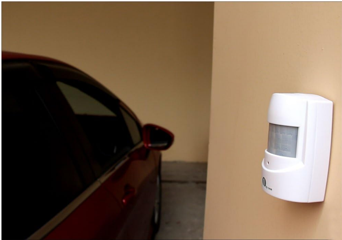
Figure 4: Example of PIR sensor mounting in a sheltered area.
