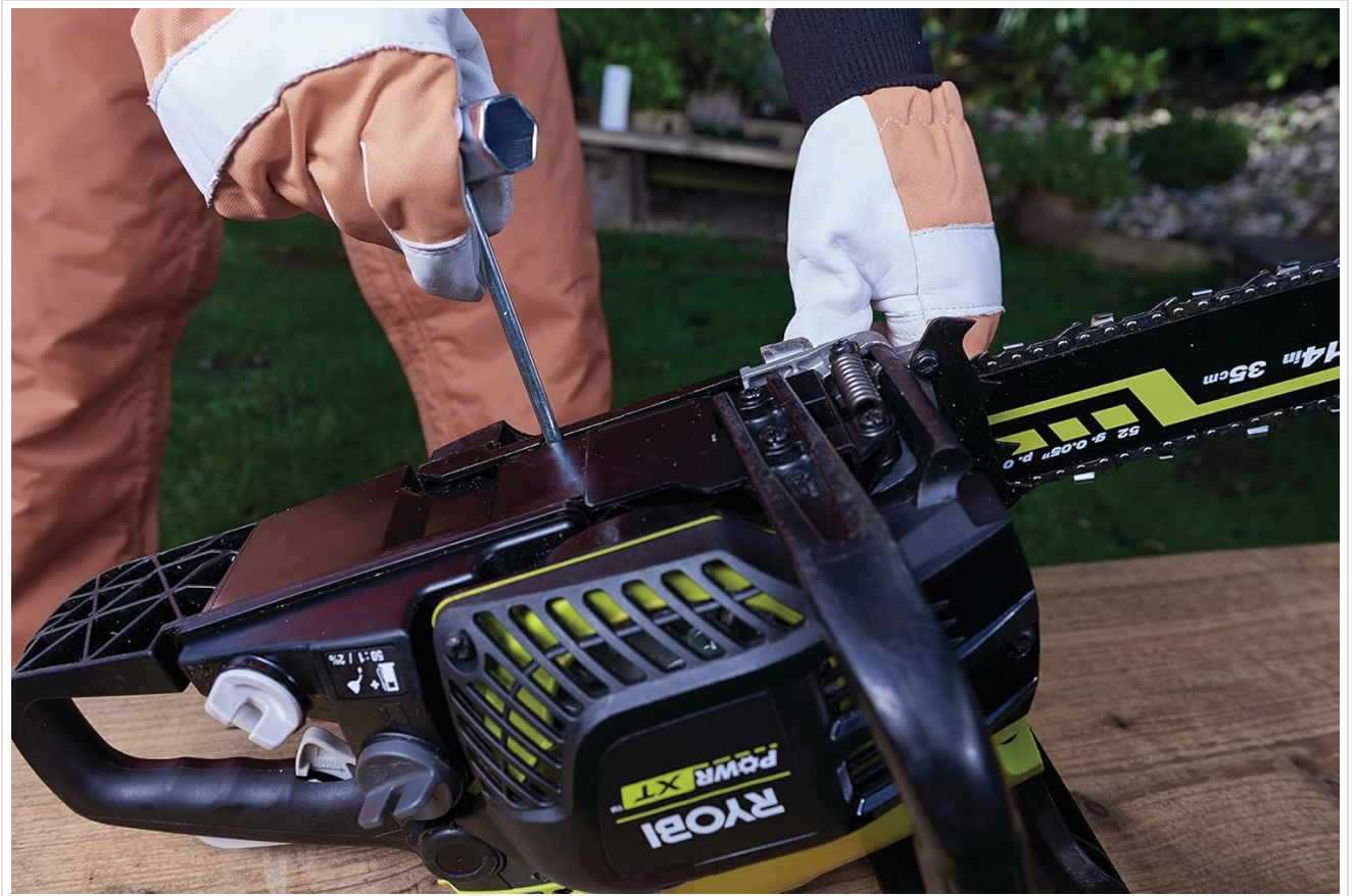
Figure 3: Utilizing the tool-free chain tensioning mechanism. This image provides a close-up view of the chainsaw's tool-free chain tensioning system, showing how to easily adjust the chain without additional tools.
