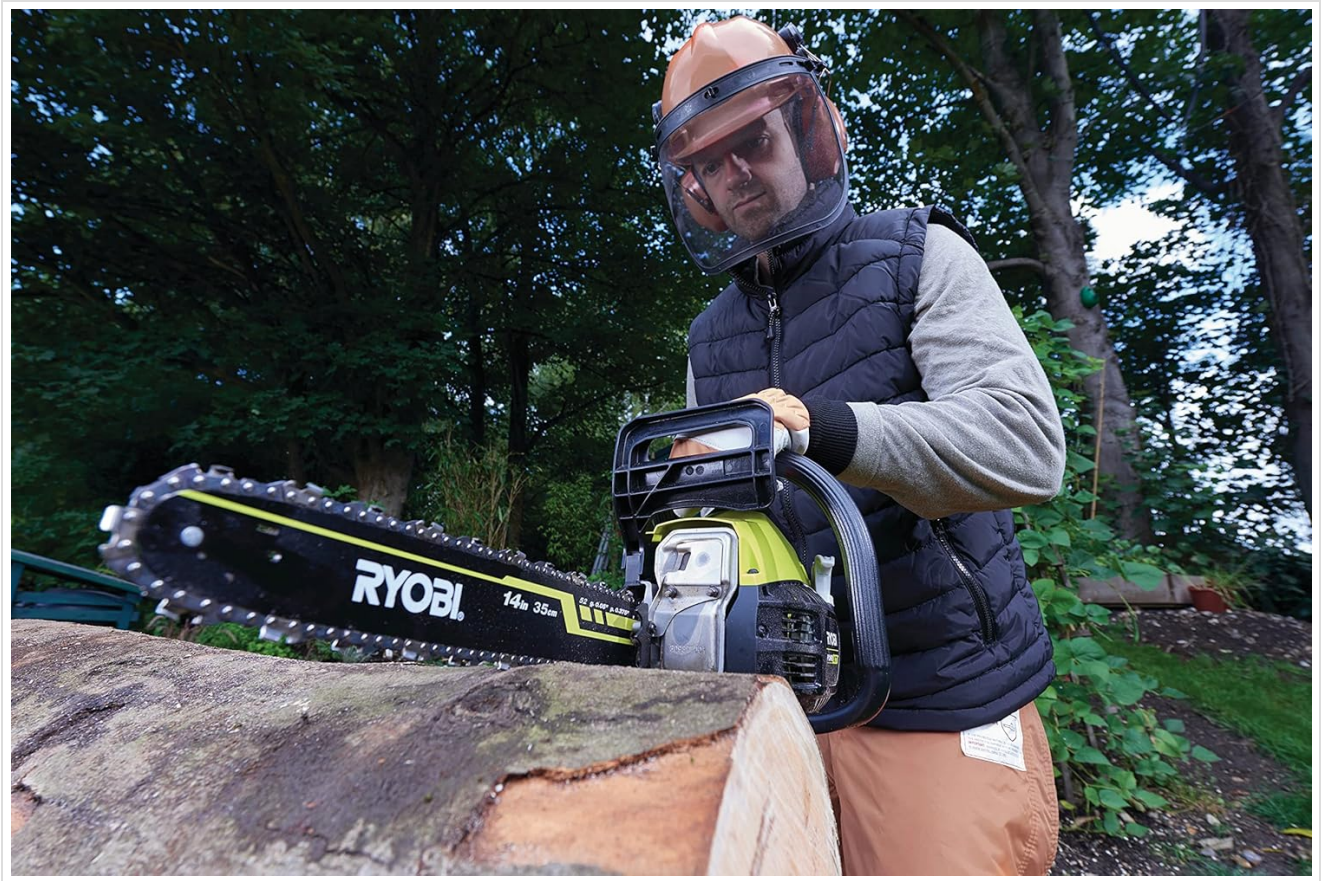
Figure 4: User operating the chainsaw. This image shows a person wearing safety gear, including a helmet with a face shield, operating the Ryobi chainsaw to cut a large log, demonstrating proper cutting posture.
