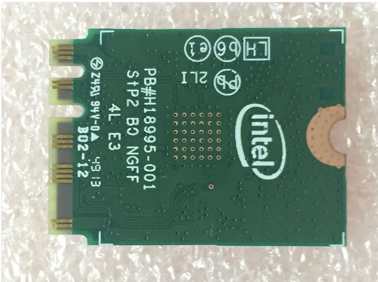
Figure 2: Bottom view of the Intel 7265NGW wireless card. This side features the Intel logo and the gold-plated NGFF connector pins that insert into the laptop's M.2 slot.
