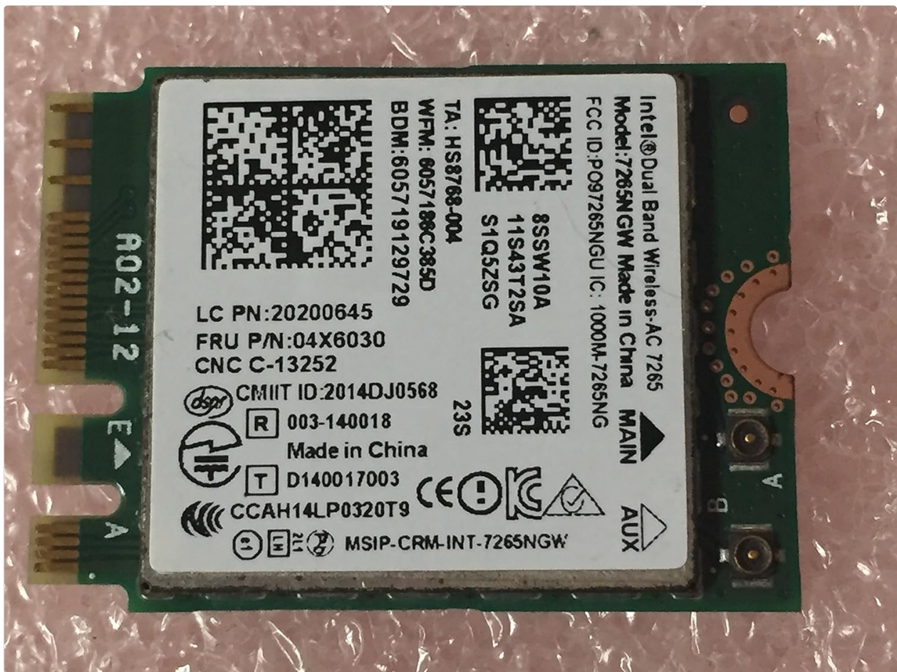
Figure 1: Top view of the Intel 7265NGW wireless card. This side typically faces upwards when installed, displaying the model number, FRU, and regulatory information.
