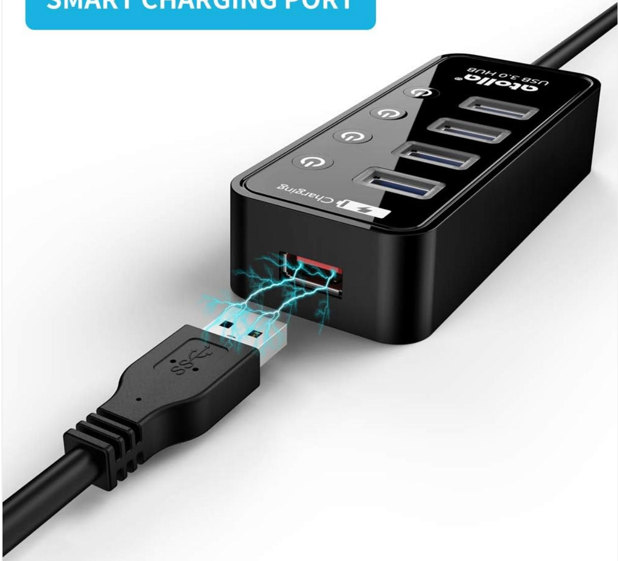
Image: A close-up of the atolla USB 3.0 Hub highlighting the dedicated Smart Charging Port, indicated by a lightning bolt icon.
