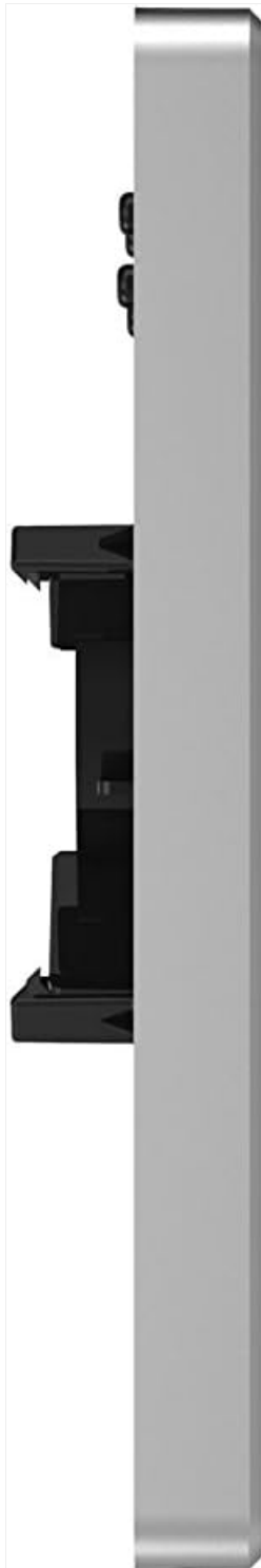
Figure 2: Side view of the Aeon Labs AL001 Touch Panel. This image illustrates the slim profile and the mounting clips designed for flush installation.
