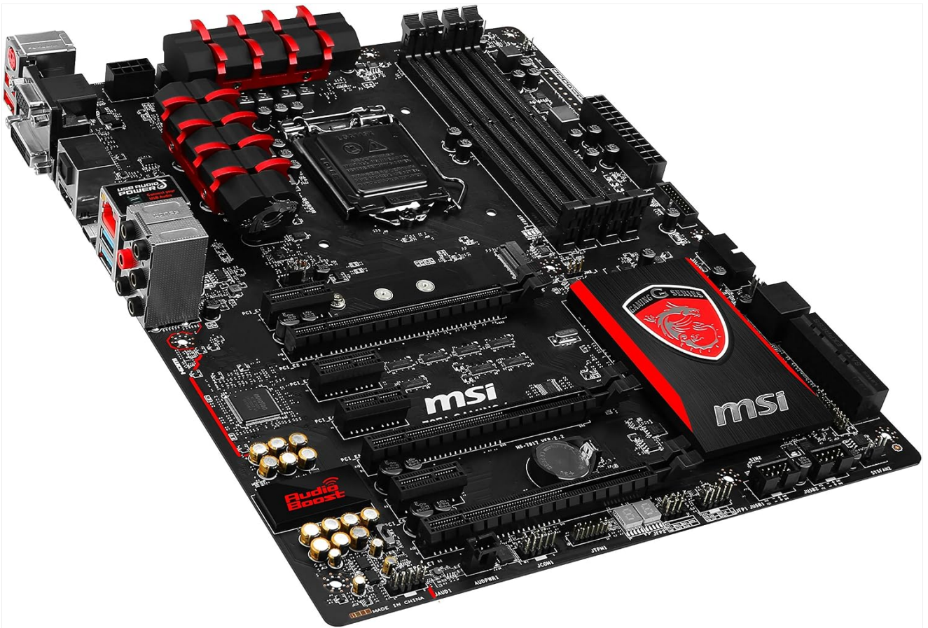
Figure 4.1: Angled view of the MSI Z97A Gaming 6 motherboard, highlighting the CPU socket, RAM slots, and heatsinks.
