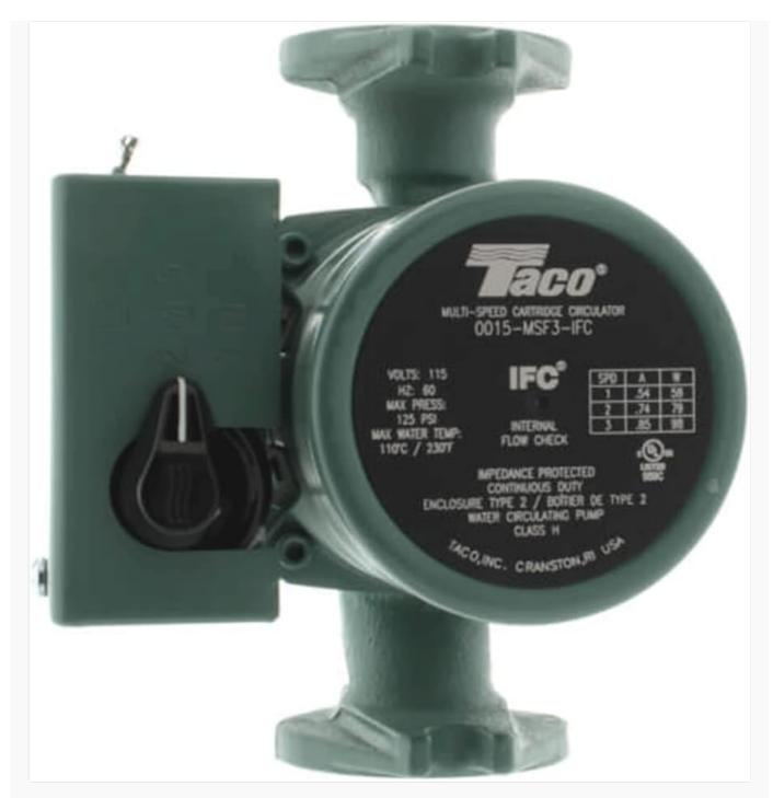
**Image Description:** A front view of the Taco 0015-MSF3-IFC circulator pump, clearly showing the product label with specifications and the speed selector switch. The label details voltage, frequency, max pressure, max water temperature, and power consumption for each of the three speeds.
