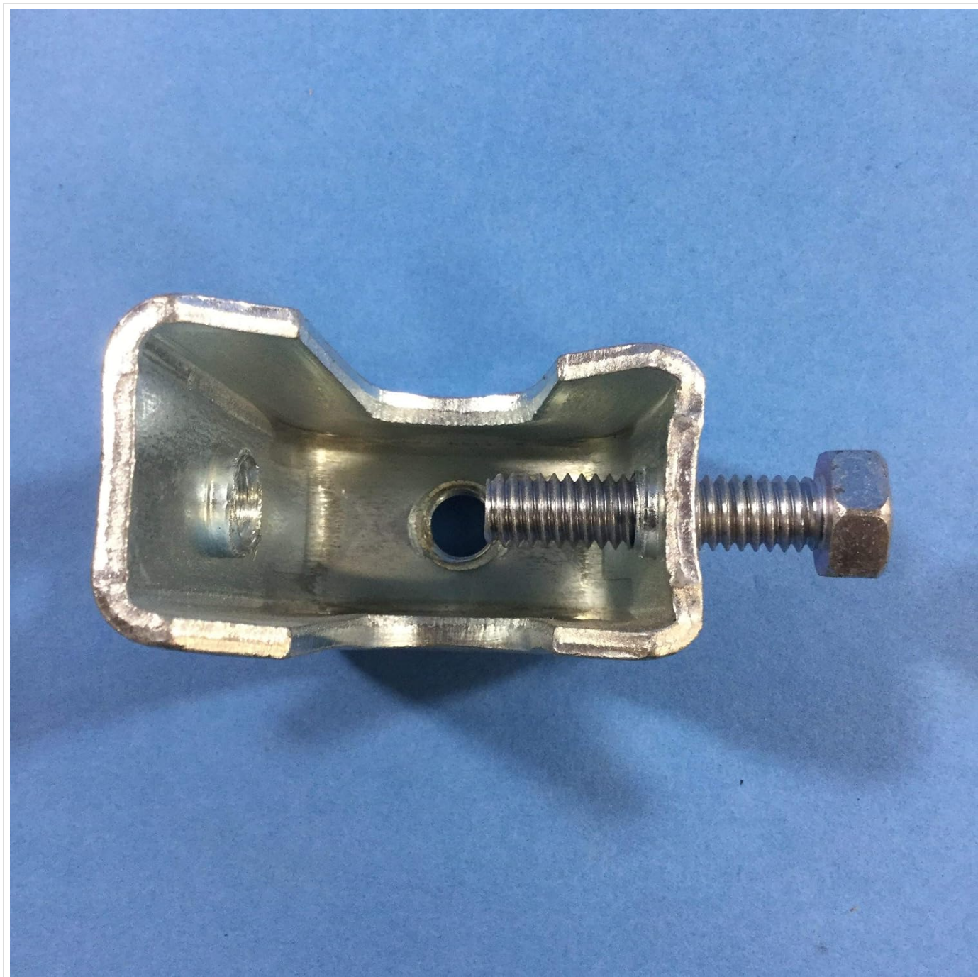
Figure 2: Top-down view of the Erico BC400 Steel Beam Clamp. This image illustrates the clamp's internal structure and the set screw mechanism, showing how it engages with the beam flange.
