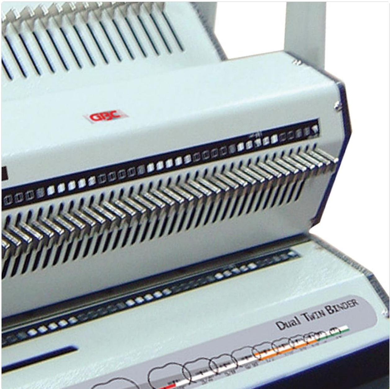
Figure 4: Close-up of the punching pins. The machine features robust punching pins for consistent hole formation.
