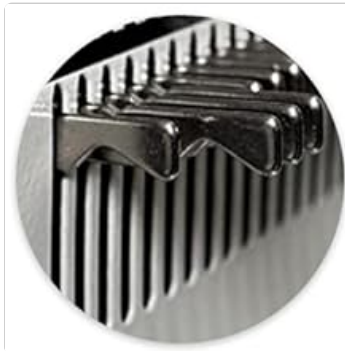
Figure 6: Close-up of the wire binding mechanism. This shows the section where wire elements are placed for closing.
