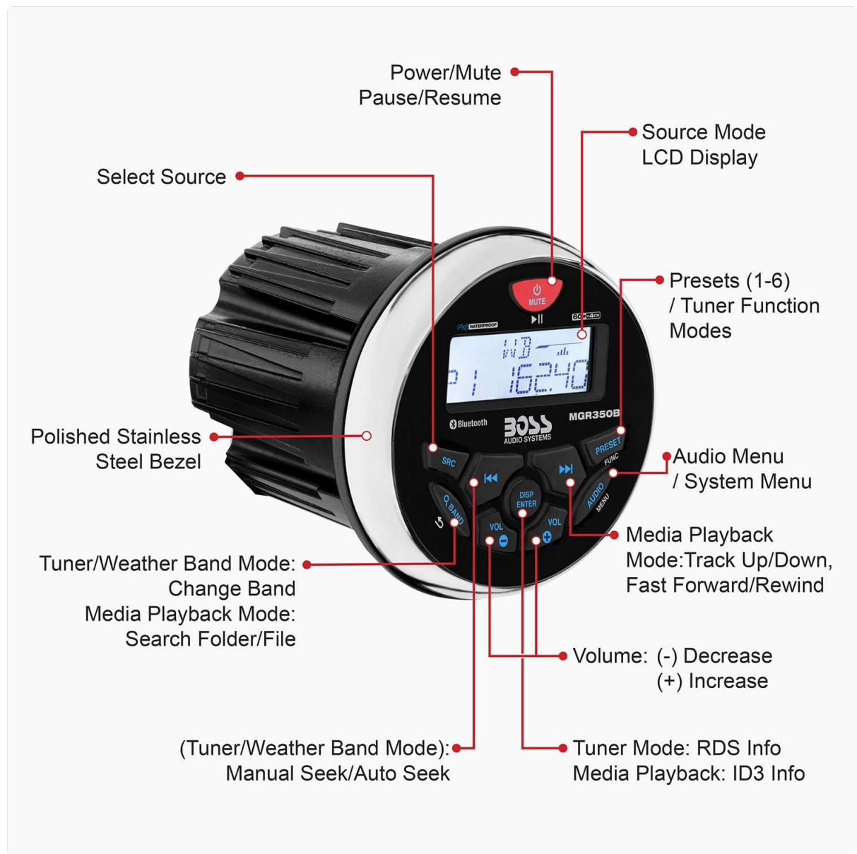
Image: Front panel layout of the MGR350B, detailing the function of each button and the information displayed on the LCD screen.
