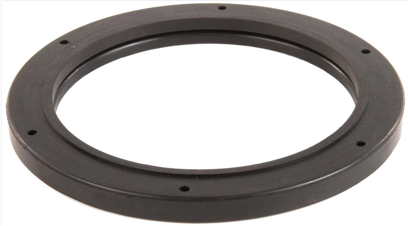
Image: The InSinkErator 11016 Mounting Gasket. This is a circular, black rubber component designed to create a watertight seal in food waste disposer installations. It features a flat, wide base with a raised inner ring and several small, evenly spaced holes around its perimeter, likely for alignment or securing purposes.
