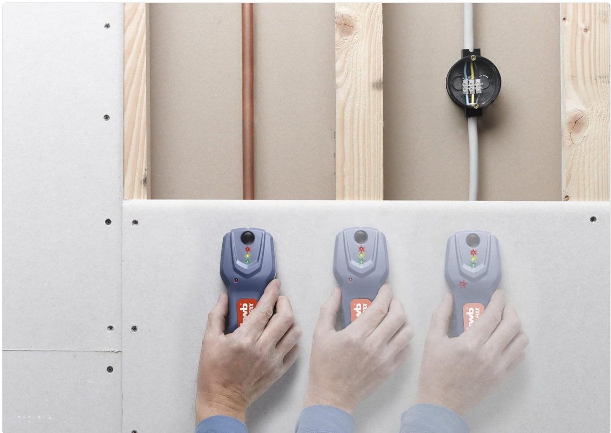
Figure 5: Illustration of detection progression as the device moves over hidden objects.
