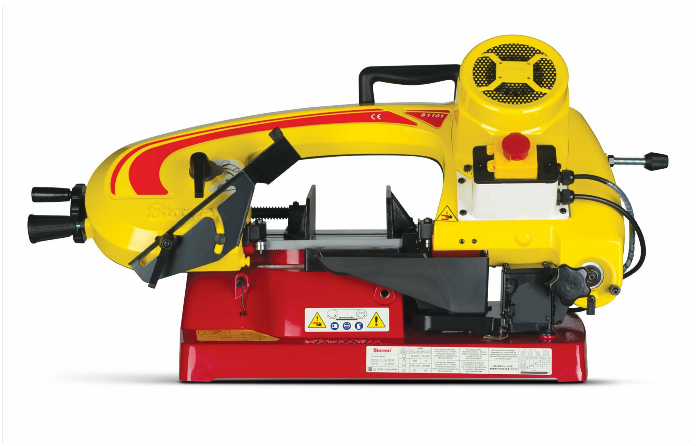
Figure 1: Starrett ST-1101 Band Saw Machine. This image shows the complete band saw unit, highlighting its compact design and robust construction, suitable for various workshop environments.
