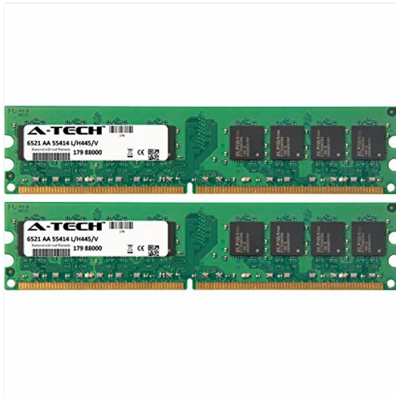
Image: Two individual A-Tech 2GB DDR2 800MHz PC2-6400 DIMM RAM modules, showing the green PCB and black memory chips.
