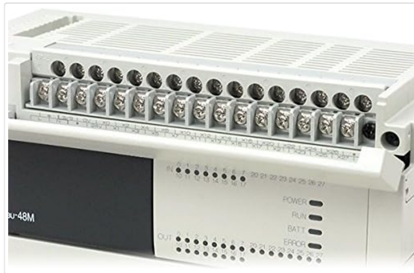
Figure 3: Close-up of the terminal blocks on the FX3U-64MR/ES. This detailed view shows the screw terminals for connecting input (X) and output (Y) wiring, along with their respective numbering, facilitating precise electrical connections.
