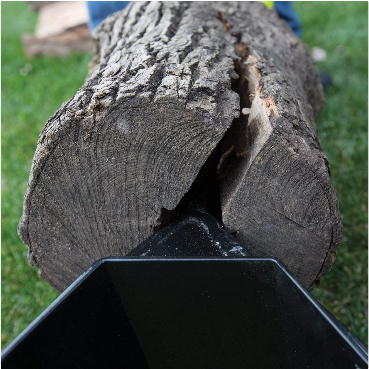
Image 5.2: A close-up view demonstrating the splitting action of the Sun Joe LJ10M, showing the wedge penetrating the log.
